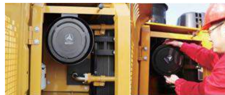
Replace air filter element
