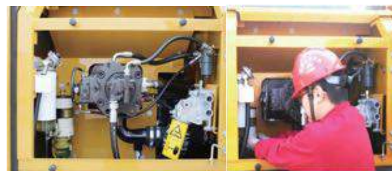
Replace diesel oil filter element
