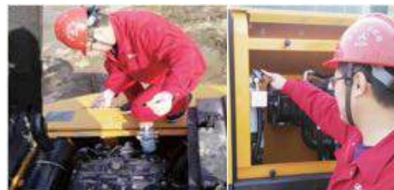
Inspect the situation of engine oil
